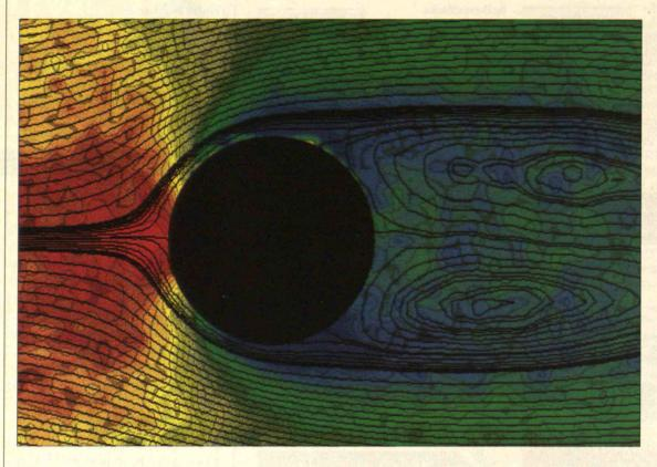
A new mathematical system, reflecting the mechanics of colliding molecules when air flows around objects, may reduce the need for extensive amounts of wind-tunnel testing. For the cylinder at left, red indicates the greatest pressure, blue the least.
