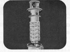
"Pull-Out" Condensate Pumps simplify maintenance because entire pumping element, including all rotating parts, can be removed without disturbing either the pump barrel or the piping connections.
