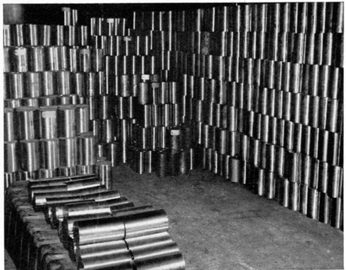
CASTING PRACTISE AT WOLVERINE IS THE RESULT OF MANY YEARS OF EXPERIMENT AND PRODUCES THESE BILLETS FOR THE EXPRESS PURPOSE OF EXTRUDING NON-FERROUS TUBES
