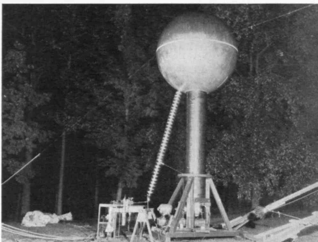
A model of the Van de Graaff generator built by Dr. Merle Tuve at the Department of Terrestrial Magnetism of the Carnegie Institution in Washington. It has a six-foot sphere and is shown with an x-ray tube connected between the terminal and the earth. Its outdoor operation has been interrupted by the bugs and fireflies drawn to the sphere
